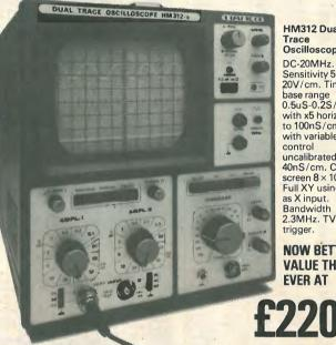
HM312 Dual Trace Oscilloscope DC-20MHz. Sensitivity 5mV-20V/cm. Time base range 0.5uS-0.2S/cm with x5 horiz mag to 100nS/cm. with variable control incalibrated to 40nS/cm, CRT screen 8 × 10cm Full XY using chil
