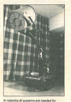
recognising objects. This mobile robot developed at Warwick University has sensory equipment enabling it to avoid obstacles and to seek out, approach and grasp an object such as the plastic bin shown.
